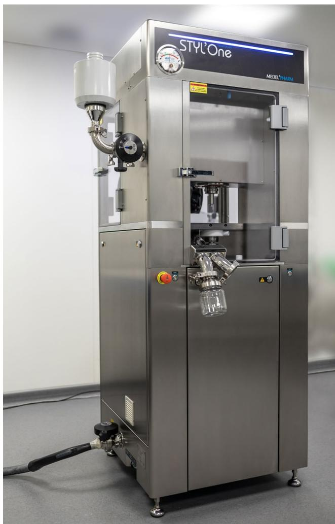
Figure 4: STYL'One EVO Multilayer R&D Compaction Simulator
